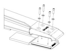
Heavy duty wear pads can be replaced while maintaining welded tip integrity.
