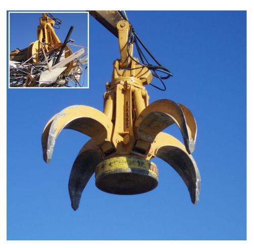
Magnet Grapples are used to clean out trailers, ground sweeping, load, unload and sort.
